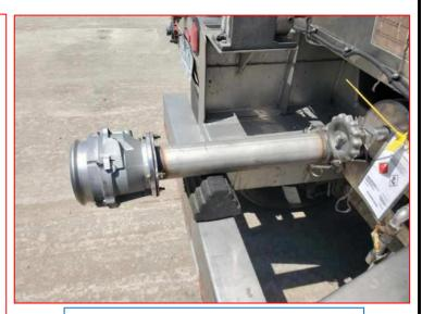
3" MALE (API) DRY CONNECTION WITH 3" QUICK CONNECT NIPPLE FITTING
