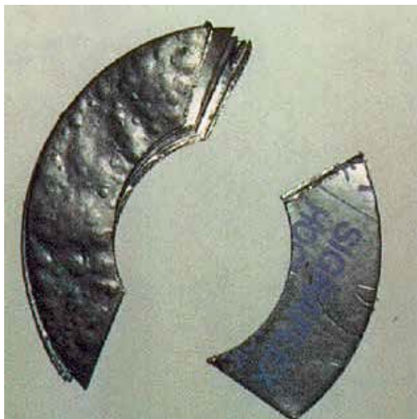
Figure 6.8 Gasket Test Showing Failure of Compressed Graphite Gasket, Laminated on Flat Stainless-Steel Sheet with an Adhesive
