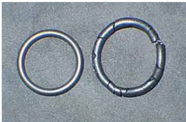
Figure 6.10 A & B Illustrates degradation of FFKM attack over time in service
