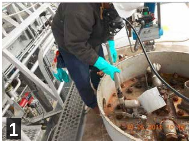
Figure 9.6 Typical steps for the transfer/unloading of Ethylene Oxide from the railcar to the receiving storage vessel.
