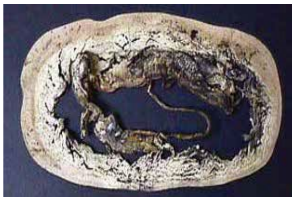
Figure 6.3 Glass Filled PTFE Gasket Failure Due to EO Polymerization in PTFE-Glass Matrix
