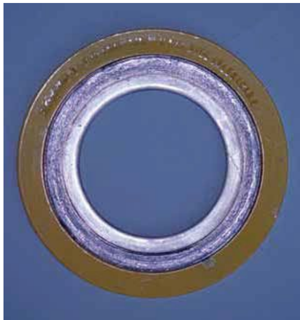
Figure 6.5 Spiral Wound Gasket with Stainless Steel Windings, Flexible Compressed Graphite Filler, and Inner and Outer Retaining Rings
