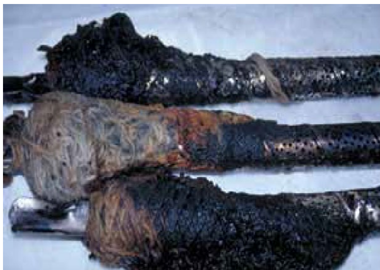
Figure 5.23 Filter Case after Runaway Polymerization
