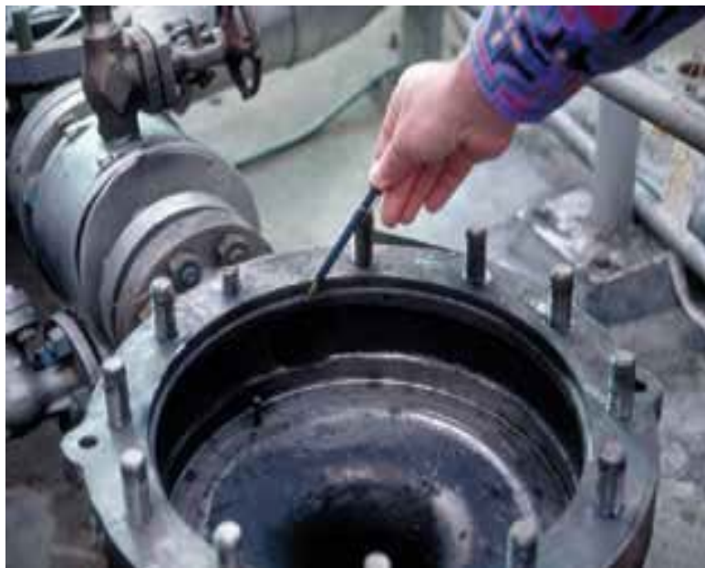
Figure 5.10 High Speed Centrifugal Pump “Launched” by Decomposition of 0.6 Pounds of Ethylene Oxide
