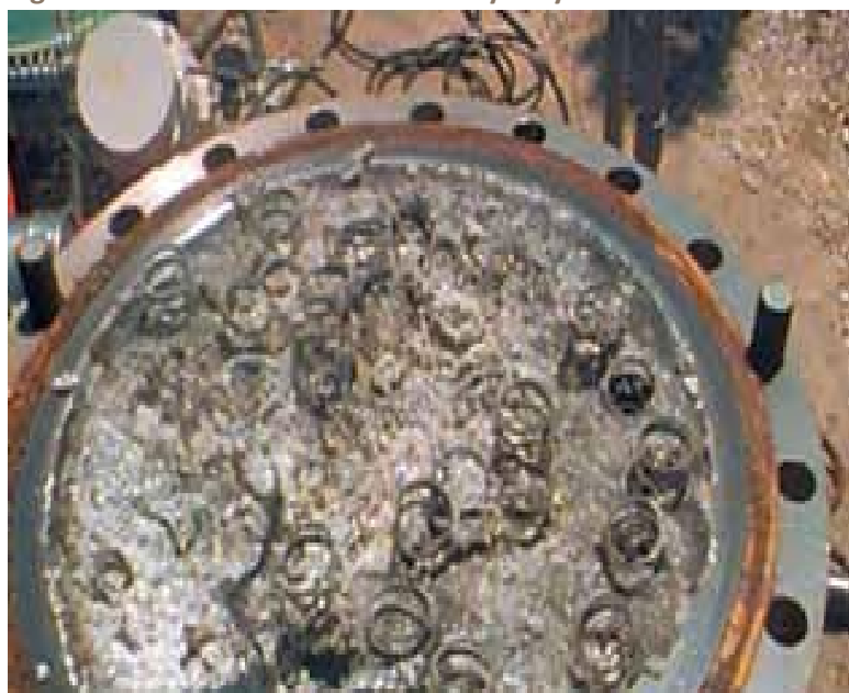
Figure 5.21 Filter Case after Runaway Polymerization
