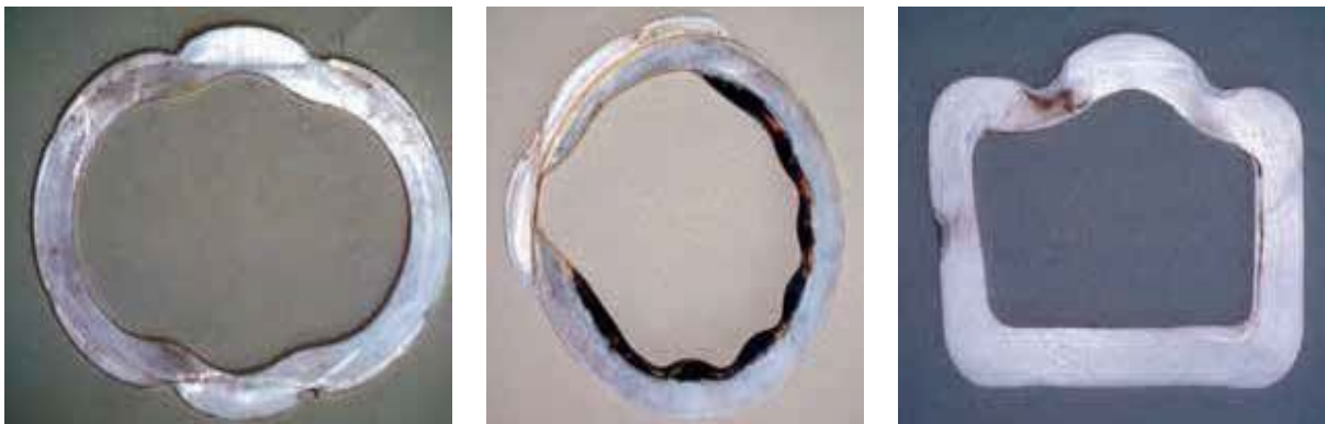
Figure 6.2 PTFE Gasket Failures in EO Service Due to Cold Flow
