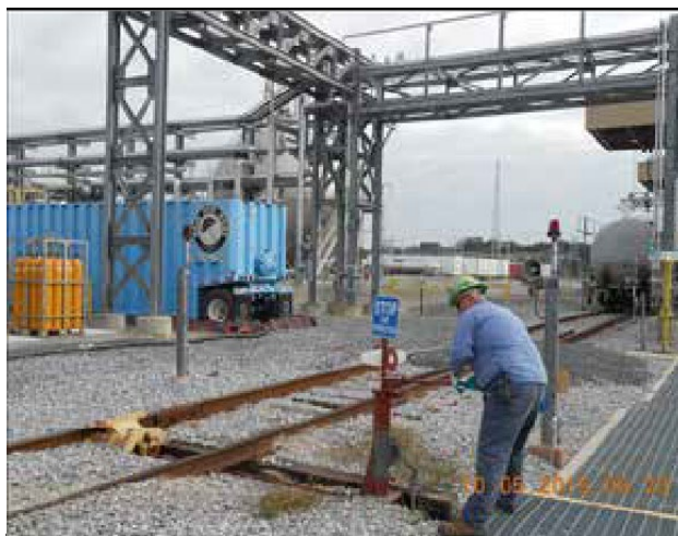
Locking track switches and utilizing a derail mechanism to prevent collisions with other cars
