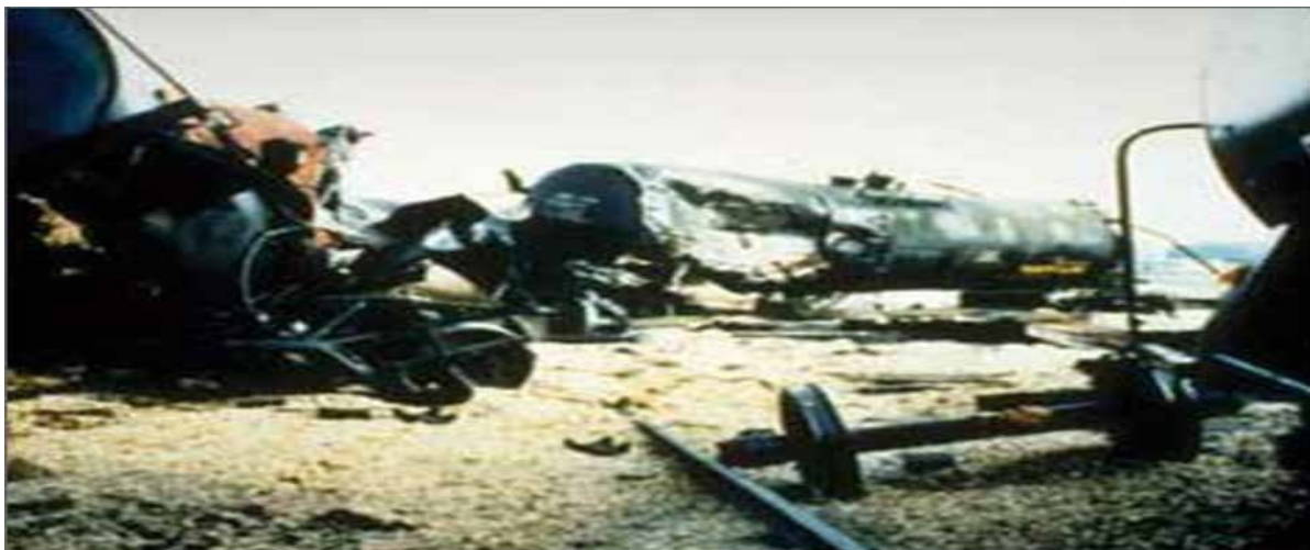
Figure 5.8 Damage to Other Railcars from Ethylene Oxide Railcar Explosion
