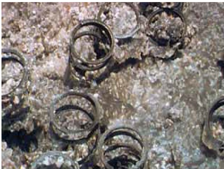
Figure 5.23 Filter Case after Runaway Polymerization
