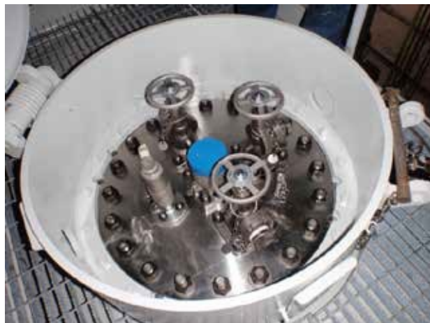
Figure 9.2 Dome Arrangement of a DOT 105- J Railcar for Ethylene Oxide Service
