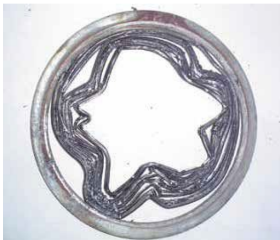
Figure 6.4b Deformation of a Spiral Wound Stainless Steel-PTFE Gasket
